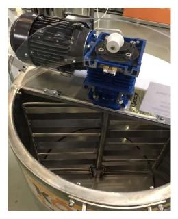
Picture 2. The drive motor with the double-winged mixing paddle
